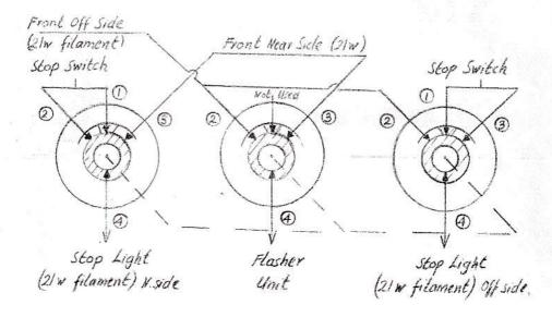
In normal position all (1)'s connect with all (4)'s and stop lights operate normally and Flashers are disconnected.
